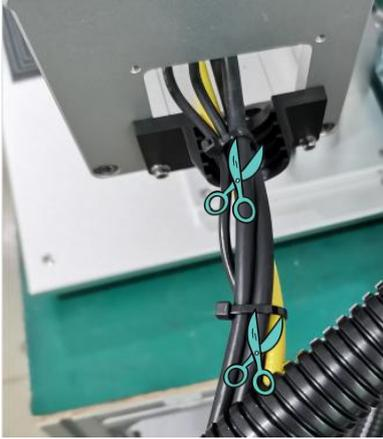
**5<sup>th</sup> Step:** Remove the cables (24V+ / 24V- / PE) on the DC24V switching power supply, then take out the laser source, as shown in the figure.
