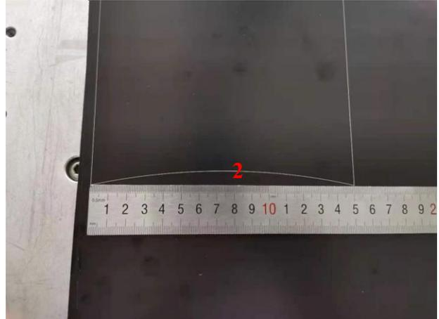
**Tip: If the line for X axis is curved toward the center, this value should in the red box be decreased; If the line for X axis is curved toward the outside, this value in the box should be increased.**
