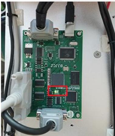
**Solution:** Restart your machine before you run the software and check the status of the light . When the machine **stands by** (including the situation that you press F1 to let the machine simulate the laser marking via red light), the light on control card shows **GREEN**; when the laser is **firing**, the light is **RED**.
