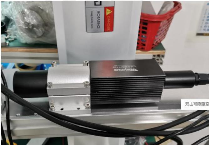
**Third Step:** Install the laser machine cavity, as show in the figure.
