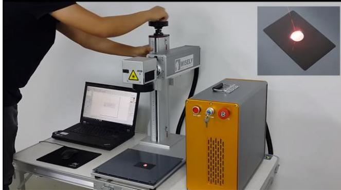
**Solution 2:** Measure the distance from the surface of objects to the middle of the scanner, then record the distance, a sticker will be of help.
