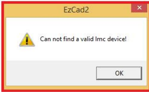
This means that the **DRIVER** of the control card might have problem or be lost, we need to check it and re-install it if necessary.
