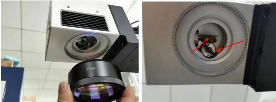
**After checking the above items, we confirm the parts are good in condition, then we can confirm that the fiber laser source is damaged, you need to send it back to us for repairing or replacement.**
