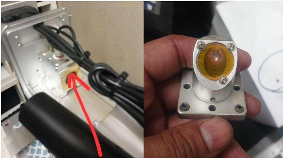
**Warning: The red light pointer is Class 3R product, you have to power off the machine before changing the Red Light Pointer.**
