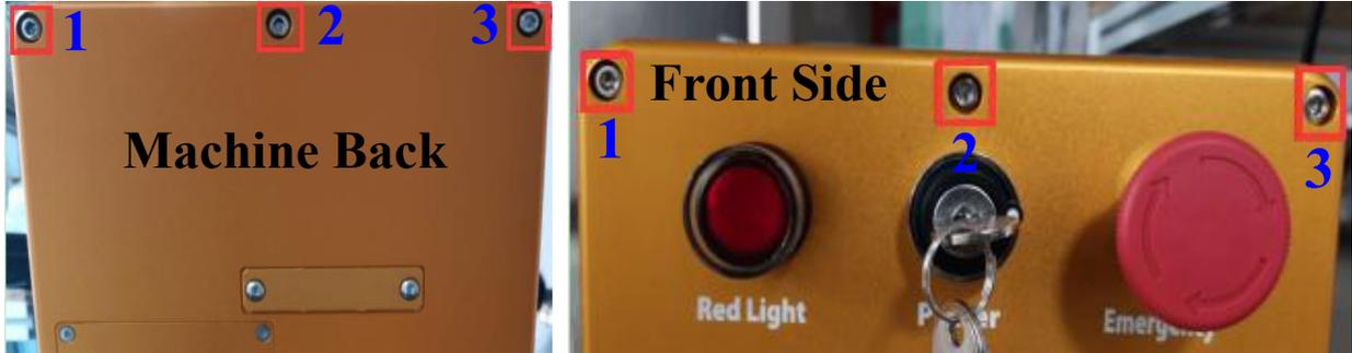
2<sup>nd</sup> Step: Disassemble the shell of the machine, as shown in the figure.
