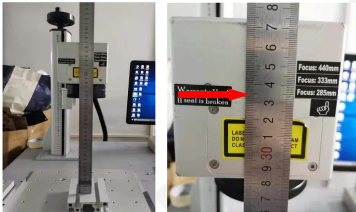
**Solution 3:** Raise or lower the Z Column until the two Red Dot Pointers are overlapping, you will see one dot only, as show in the figure.
